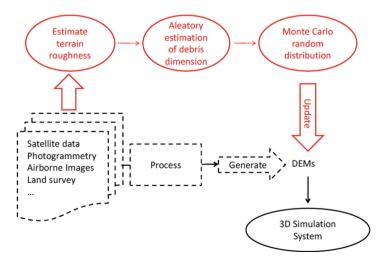
Fig. 7. Enhanced input integration process (DEM based example).
