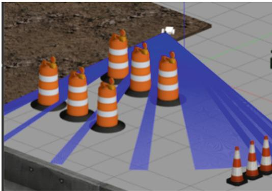
**Fig. 3.** Example of Sensor (LIDAR) model - Global view
