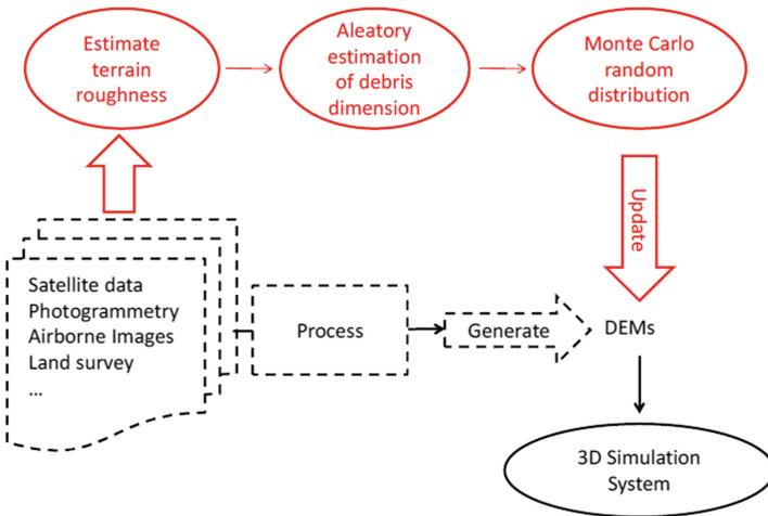
Fig. 7. Enhanced input integration process (DEM based example).
