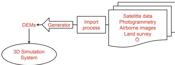
**Fig. 5.** Terrain input process to simulation system
